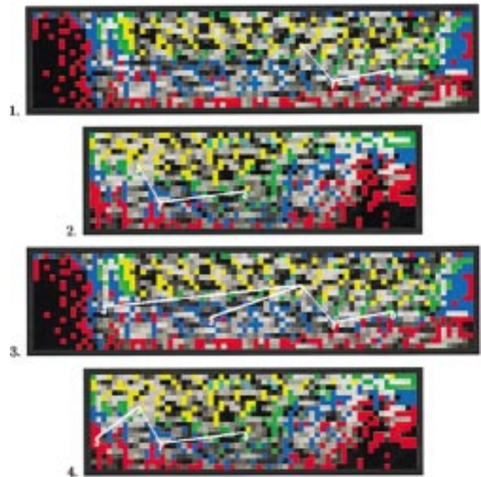
Fig. 4. 1) Graph on a digit “4” at node 011 in the tree used in Table I. 2) Graph on a digit “1” at same node. 3) Graph on the same digit “4” at node 01111 in the same tree. 4) Graph on same digit “1” at node 01110 in the same tree. Each colored pixel denotes a tag (Fn, Qm) , n = 1, \dots, 18 , m = 0, \dots, 8 . The frequency channel associated to a tag is read by the row number (from top to bottom) in the spectrogram. The energy quantile is coded by four colors. We have paired consecutive quantiles due to graphical constraints. Red: Q0,Q1, blue: Q2,Q3, green: Q4,Q5, yellow: Q6,Q7, cyan: Q8.
