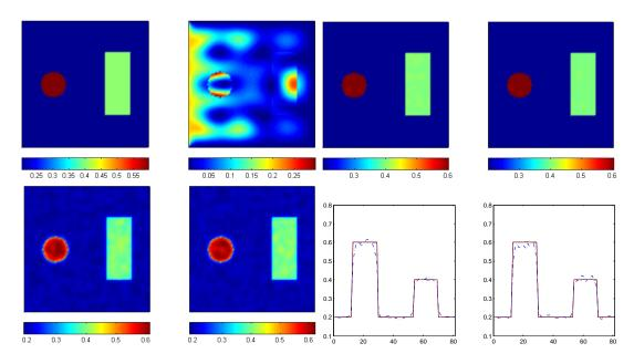
Figure 1. Reconstructions of an conductivity profile. From top left to bottom right: true conductivity, measurement  $\sigma |u|^2$ , reconstructed conductivity with first and second method with noise-free data, reconstructed conductivity with first and second method with noisy data, and the cross-sections of true (solid) and reconstructed (red dashed and blue dot-dashed)  $\sigma$  along y = 1.0
