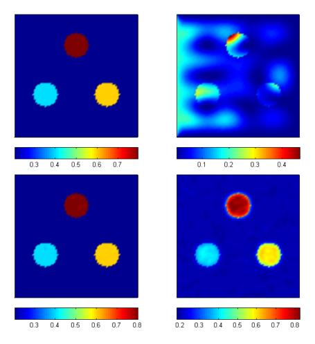
Figure 3. Reconstructions of an conductivity profile for the vectorial Maxwell equation. Top row: true conductivity and measurement  $\sigma |E|^2$ ; Bottom row: conductivities reconstructed with noise-free data and noisy data.
