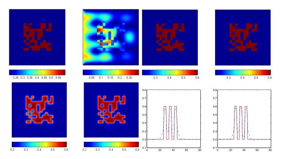
Figure 2. Reconstructions of an conductivity profile. From top left to bottom right: true conductivity, measurement  $\sigma |u|^2$ , reconstructed conductivity with first and second method with noise-free data, reconstructed conductivity with first and second method with noisy data, and the cross-sections of true (solid) and reconstructed (red dashed and blue dot-dashed)  $\sigma$  along y = 1.0
