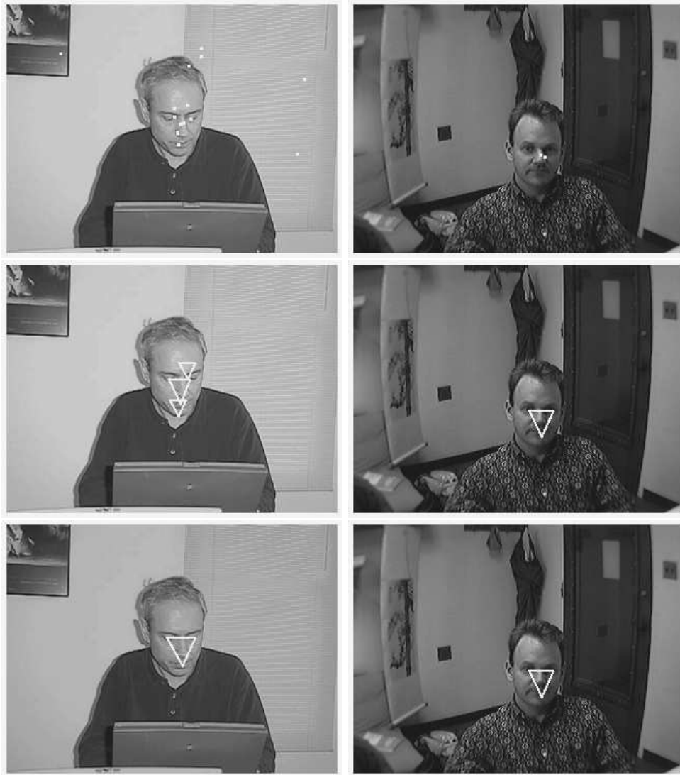
Figure 8.6: Top: Detections from step I. Middle: Detections from step II. Bottom: Detections remaining after final classifier. Detection triangles - mapping of the reference points into the image by a .
