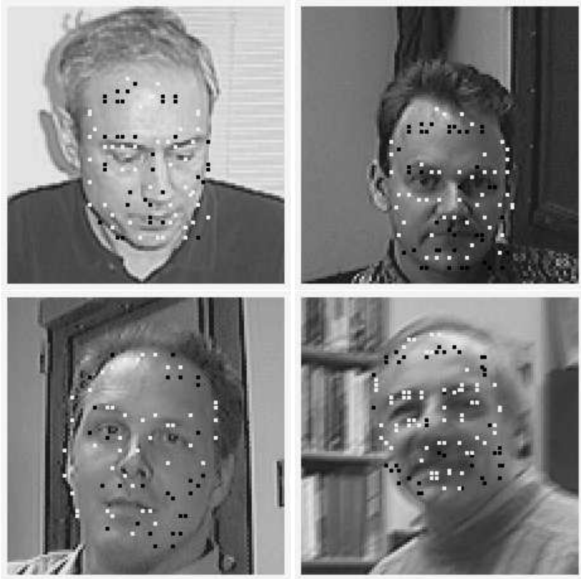
Figure 8.8: Estimated instantiation \theta on the four faces detected above. White dots show detected edge features, black dots show extrapolated features.
